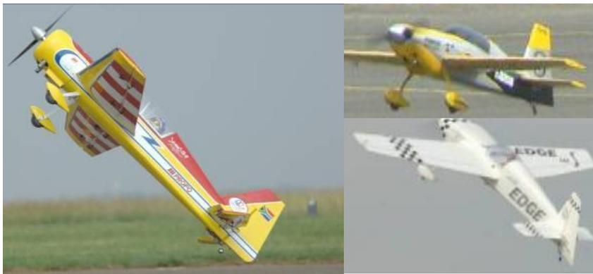
Shaun and Allen Frazer put on an impressive demonstration of their 1/3 scale YAK 54. This aircraft has a 2 cylinder petrol engine of 106 cc.
